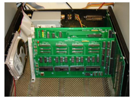
Constructing the H8-4 is very easy. Just follow the silkscreen layout for placing the parts. Be careful with the 7912 negative 12V regulator when soldering the bypass strap - voltage-in is the middle pad and voltage-out is the pad to the right. Use a half-can 1.8432MHz oscillator for timing. The hardest components to find will be the 74LS242 buffer chips. I recommend using <u>BG Micro</u> for ordering these chips.
