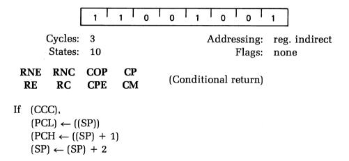
If the specified condition is true, the actions specified in the RET instruction (see above) are performed: otherwise, control continues sequentially.
